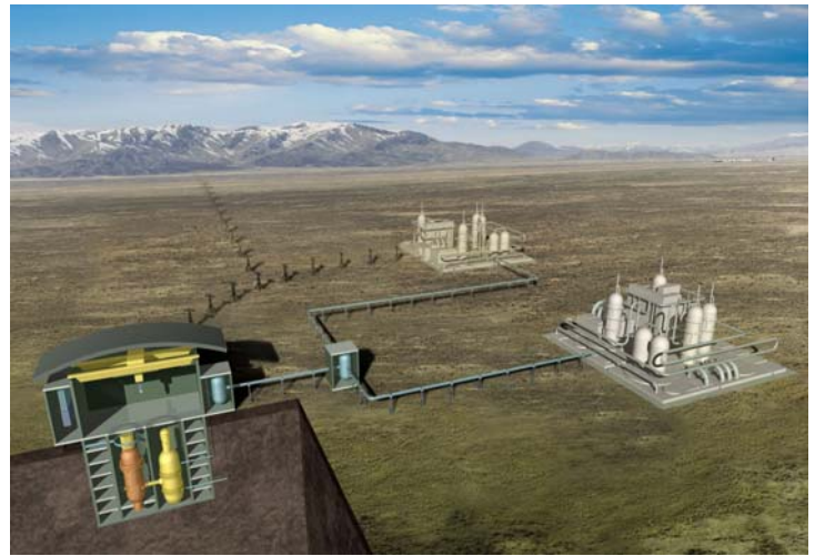
Figure 1. Potential Layout of VHTR for Hydrogen Production.
